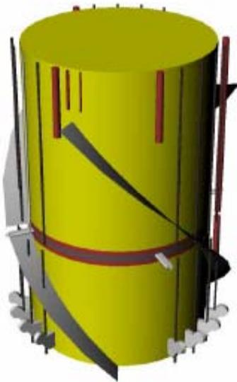
**Figure 3 - 3D view of the truss spar hull CAD drawing (Case SPC)**
