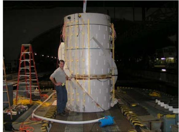
**Figure 1 - Large scale spar hull with all appurtenances (Case SPAC).**
