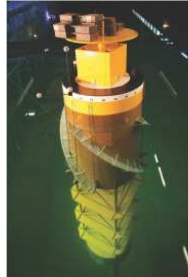
Figure 2 – Spar Tested with Four-Start Strakes
