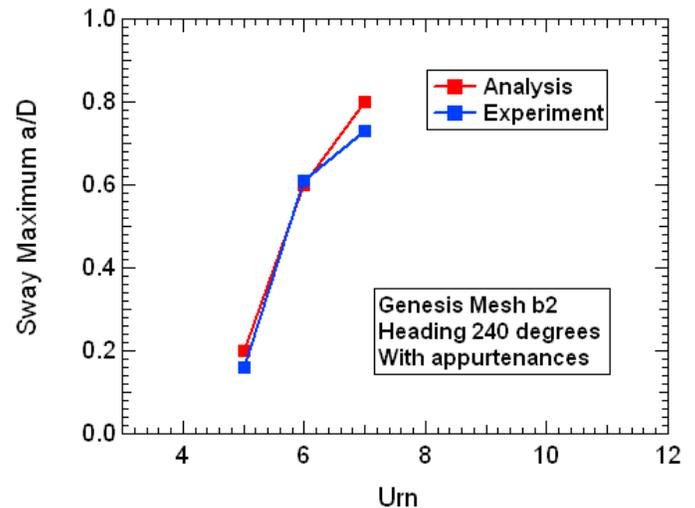
Figure 7  $a/D$  versus reduced velocity  $U_{rn}$ , uniform current model scale. The mesh includes all hull appurtenances, except for the anodes. This particular model test, unlike most others,
