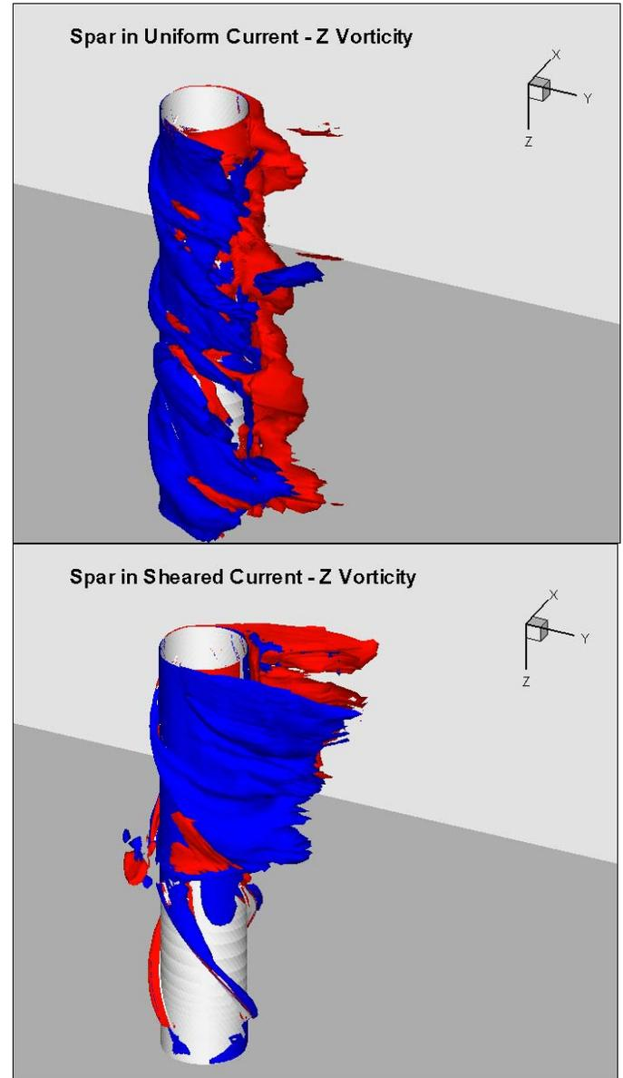
Figure 10 Flow in uniform and sheared current
