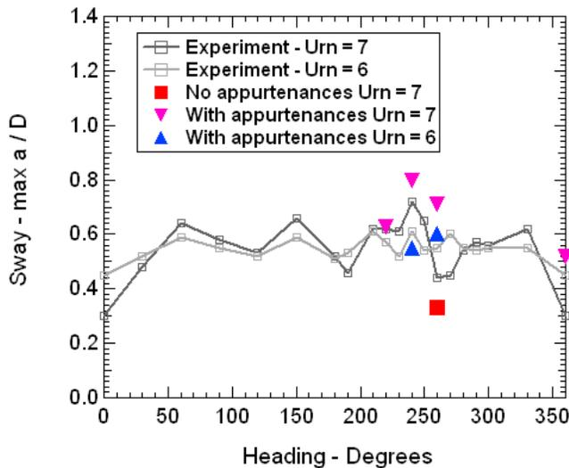
Figure 8 Spar VIM vs. heading at model scale in a uniform current profile.
