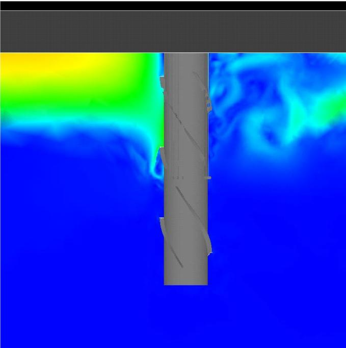
Figure 12 Predicted velocity magnitude contours on center plane for a full scale spar in hurricane currents
