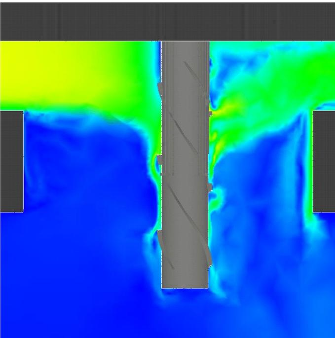
Figure 13 Predicted velocity magnitude contours for a 1:46-scale spar in a divided tank without buoyancy effects
