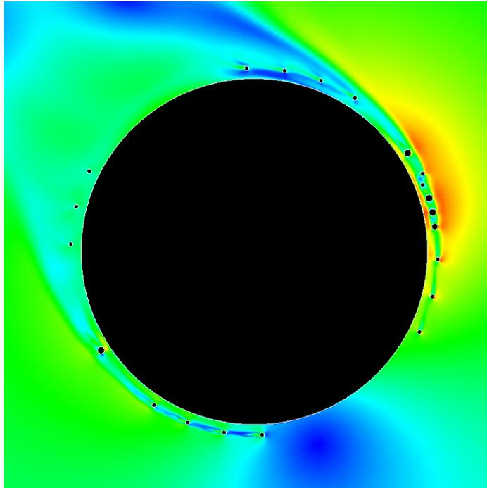
Figure 5 Influence of appurtenances on the flow around the platform as shown by velocity magnitude contours.
