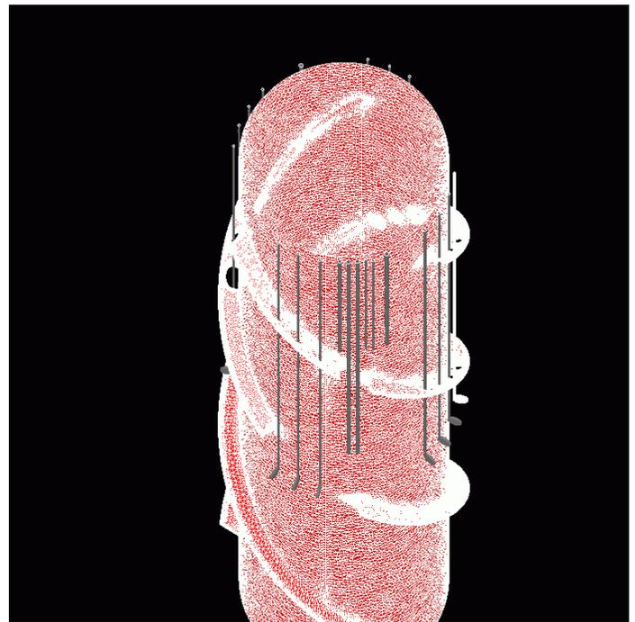
Figure 4 Surface mesh representing a spar platform with appurtenances shown in grey.
