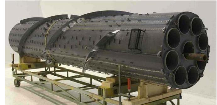
Figure 2 View from of scale model of Genesis hull as tested. The top of spar is on the right. Note strake, pipe, chain and anode details. The scale factor is 1:46.
