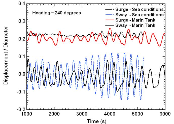
Figure 14 Comparison of  $a/D$  computed for full scale and model scale spars.
