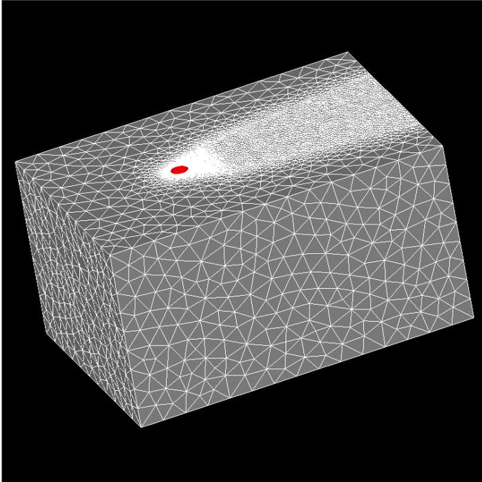
Figure 3 Surface mesh on exterior of fluid domain
