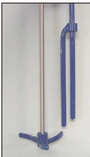
constructed for testing in a 6-in.-dia. (152 mm) vessel. The experiments were carried out with water and a glycerin-type fluid, with two different impeller shaft speeds in baffled and unbaffled configurations. The tests were observed using a particle image velocimetry (PIV) system. Experimental data were taken at several horizontal
