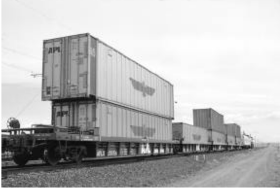
Figure 1. Generic double stack container car with containers
